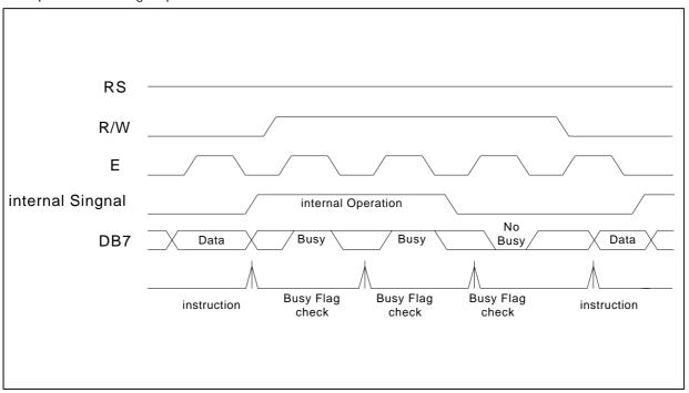
Example of 8-bit bus mode timing diagram
