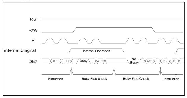
Example of 4-bit bus mode timing diagram
